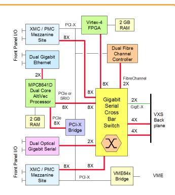
Figure 3. Model 4207 VXS I/O Processor bas dual PMC/XMC sites, dual core PowerPC, FPGA, Fibre Channel controller and Gigabit Serial Crossbar Switch that joins all of the board's resources.
