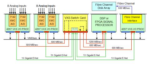
Figure 4. VXS-based 16-channel Beamforming Signal Processing and Recording System.
