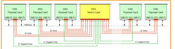
Figure 2. Switched VXS star backplane with Switch Card provides two duplex 2.5 GB/sec 4X ports for each Payload Card. Gigabit Ethernet-X ports replace VMEbus as the system control plane.
