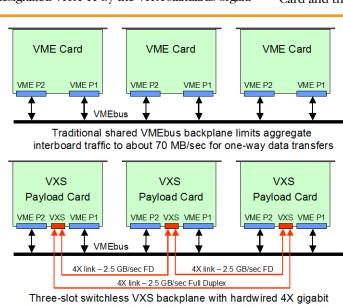
links delivers full-duplex 7.5 GB/sec aggregate interboard traffic Figure 1. VXS offers a significant boost in data bandwidth between boards.
