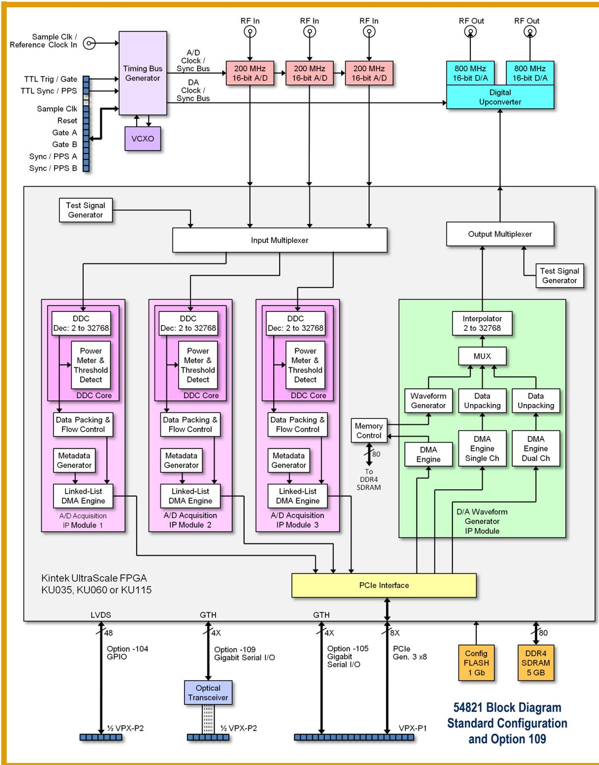
supporting PCI Express Gen. 3 as a native interface, the Model 54821 includes optional high-bandwidth connections to the Kintex UltraScale FPGA for custom digital I/O.
