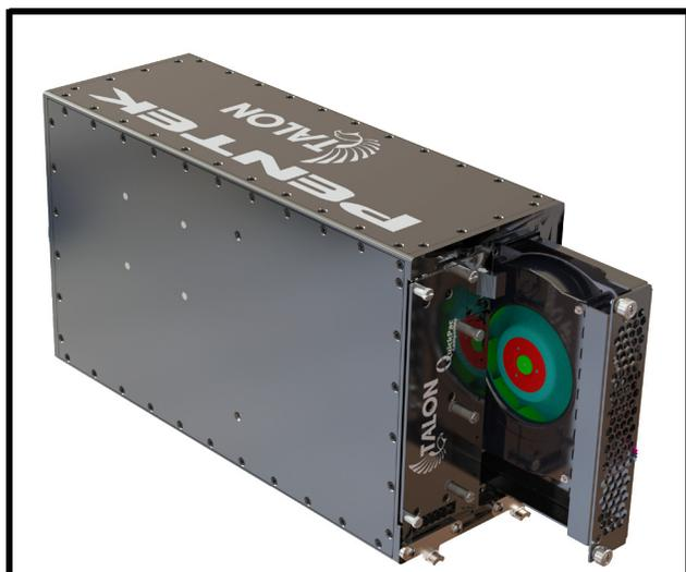
The Talon RTX SFF chassis seals the internal electronics from the outside environment by providing an inner plenum that is designed to extract heat from the internal electronics via conduction. The plenum is supplemented by a removable fan.
