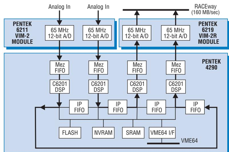
Figure 3. Quad C6201 DSP with VIM Mezzanines for A/D and RACEway
