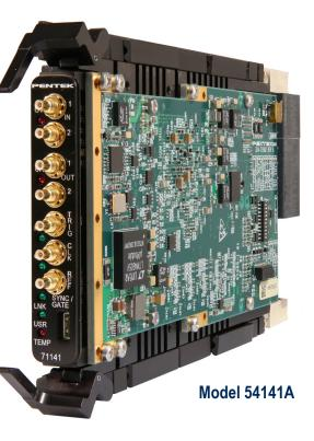
The Model 54141A supports the emerging VITA 66.5 optical interconnect standard by providing four optical duplex lanes to a mating spring-loaded backplane connector. With the installation of a serial protocol like 10 or 40 Gigabit Ethernet in the FPGA, the interface enables highbandwidth digital communications between boards or chassis independent of the PCIe interface.
