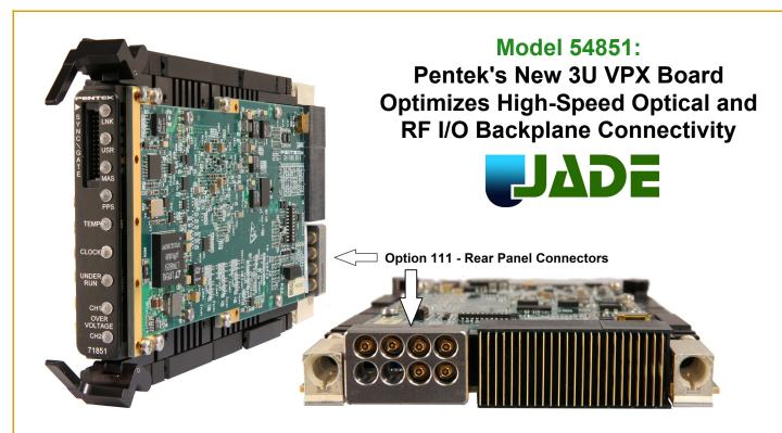
Based on the Xilinx Kintex Ultrascale FPGA, Pentek's **Model 54851** features two 500 MHz 12-bit A/Ds with two programmable multiband digital downconverters (DDCs) and one digital upconverter (DUC) with two 800 MHz 16-bit D/As. The 54851 is the first board utilizing this new 3U VPX architecture with advanced wideband I/O options.
