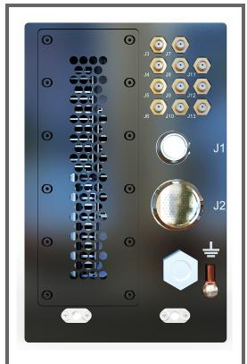
Figure 8. The Talon RTX Model 2586 recorder's rear panel connectors
