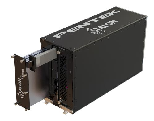
Figure 2. Pentek's QuickPac<sup>TM</sup> drive pack provides up to 30 TB of solid state storage in a small package. These pictures show the QuickPac drive pack and OS drive removed and partially ejected from the Talon Model RTX 2589 3.6 GS/ sec Ultra Wideband RF/IF Extreme 1/2 ATR Recorder.
