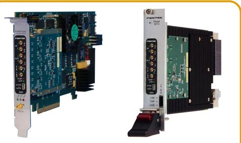
Figure 1. Models 7070-320 PCIe and 5973-320 3U VPX. Two wideband analog I/O modules featuring dual 3 GHz 12-bit A/Ds, dual 2.8 GHz 16-bit D/As, Virtex-7 FPGAs, and DMA engines supporting PCIe Gen 3 x8 PCIe data links to system memory.
