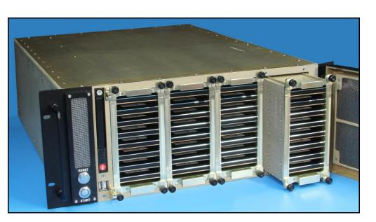
**Figure 2.** Pentek RTX 2766 ruggedized airborne recorder features four removable, hot swap QuickPac<sup>®</sup> drive packs, each containing eight SSDs in RAID arrays for easy transport of up to 60 TB of recordings to a secure facility.
