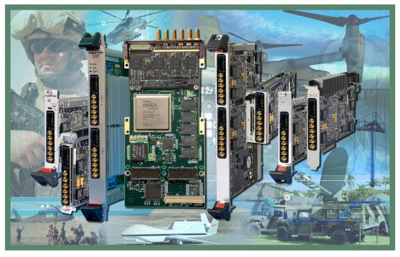
All Jade modules are available in XMC, PCIe, 3U/6U VPX, AMC, and rugged versions.
