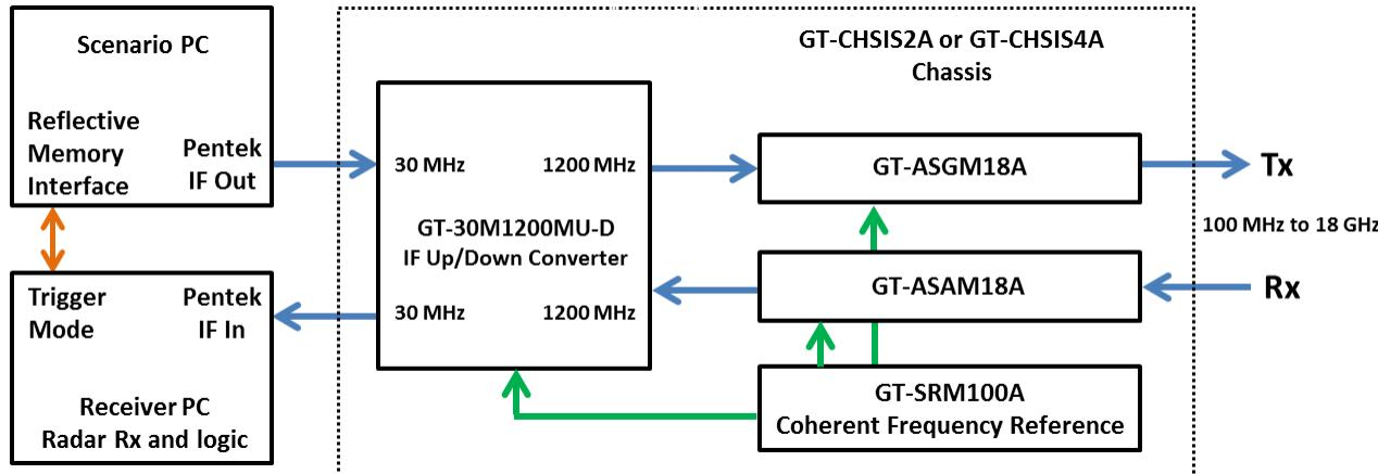
Figure 4. System Block Diagram Showing an IF Up and Downconverter
