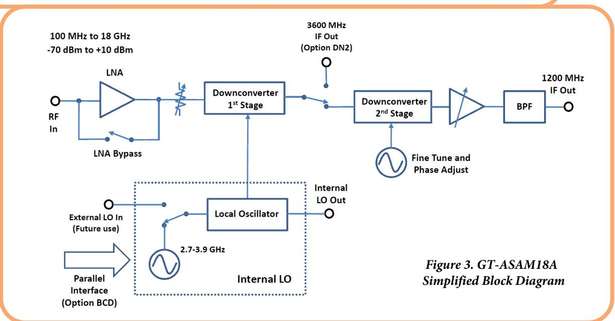
Figure 3. GT-ASAM18A Simplified Block Diagram
