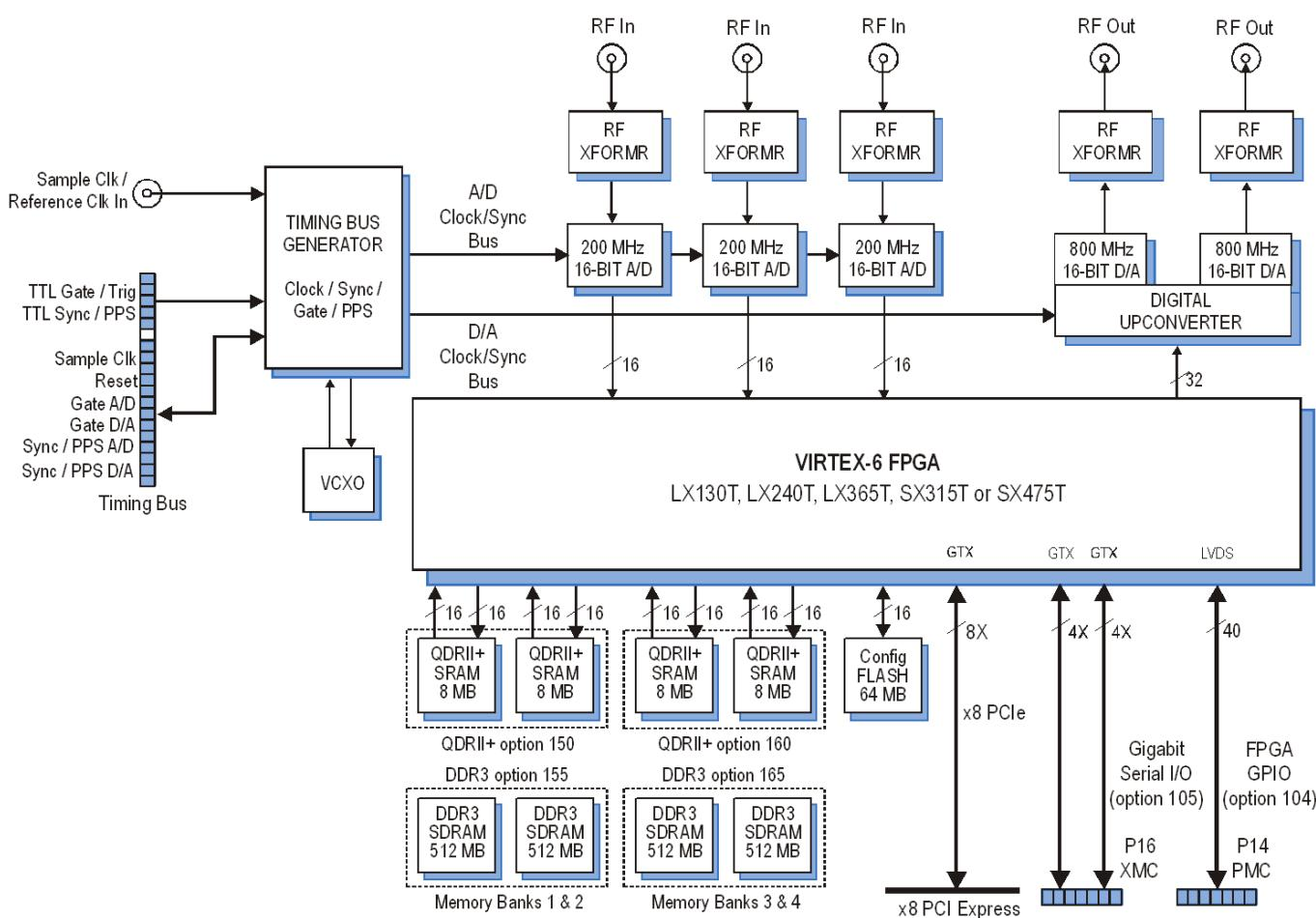
Figure 1. Pentek Model 78620 Block Diagram
