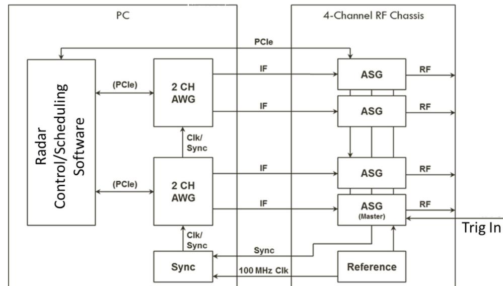
Figure 5. Radar Simulation System Block Diagram
