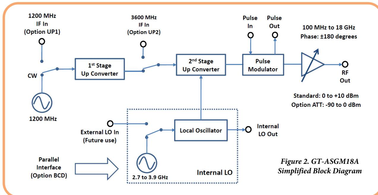
Figure 2. GT-ASGM18A Simplified Block Diagram
