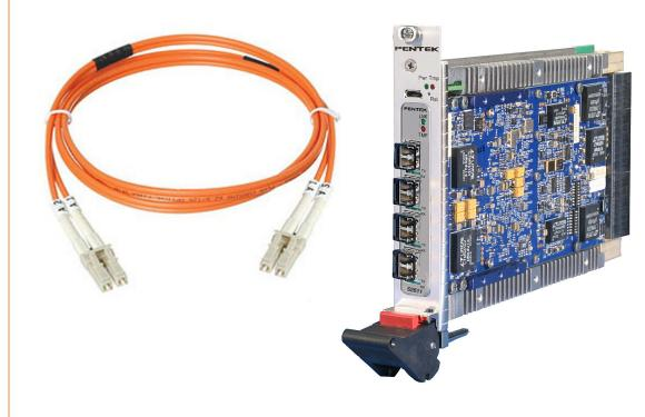
*Figure 1. <u>Pentek's Cobalt \* Model 52611 Quad Serial FPDP 3U VPX module</u> supports four full-duplex LC optical cables for connections between chassis, each operating at over 400 MB/sec*
