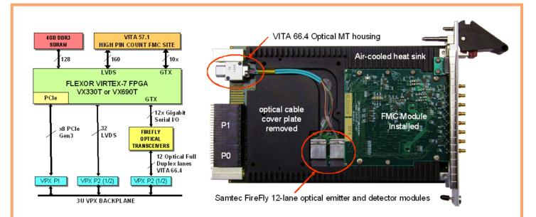
*Figure 3.* <u>Pentek's Flexor Model 5973 3U VPX Virtex-7 FMC carrier</u> is the industry's first VITA 66.4 optical backplane product. Samtec FireFly optical transceivers deliver data rates up to 12 GB/sec full duplex to the backplane supporting a wide range of protocols implemented within the FPGA.
