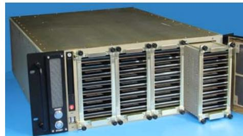
*Figure 4. Chassis View showing one QuickPac canister partially withdrawn.*
