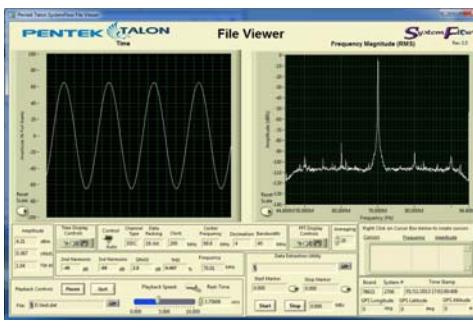
Pentek's [SystemFlow Simulator](#) for Talon analog and digital recording systems includes a virtual recorder server application that simulates disk and I/O transactions for a complete and realistic recording environment.
