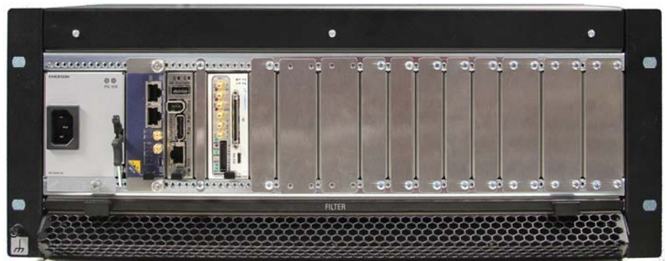
Figure 3. Typical 12-slot MicroTCA Shelf
