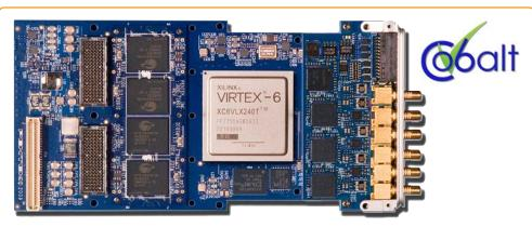
Pentek XMC Software Radio Board with Virtex-6 FPGA
