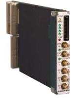
Model 7153 is also available in PCI, PCIe and cPCI formats
