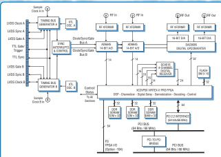
Model 7340 Block Diagram; Model 7240 contains twice the resources shown here
