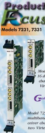
Pentek Introduces cPCI Multiband Digital Receivers: Up to 32 channels with 14-bit 100 MHz A/Ds and FPGAs
