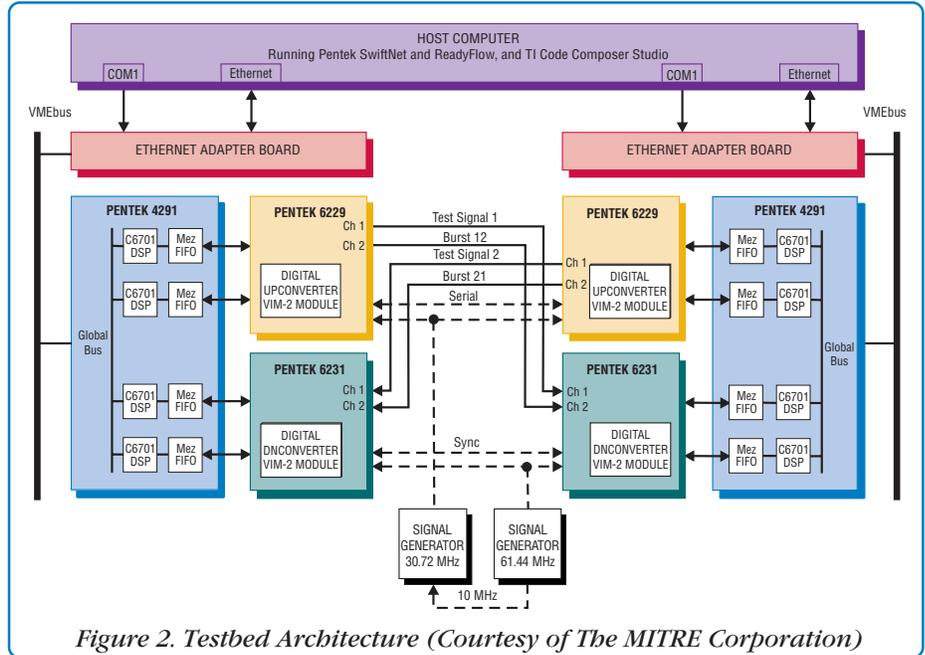
Figure 2. Testbed Architecture (Courtesy of The MITRE Corporation)
