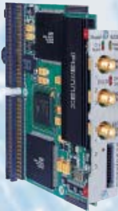
Model 6235 is a dual wideband receiver VIM-2 module that includes 12-bit 100 MHz A/Ds and a Virtex-II FPGA.
