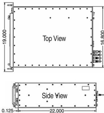
Figure 3. Dimensional drawings of the rackmount enclosure.
