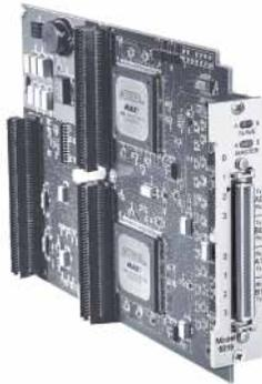
One VIM-2R plus one VIM-2 module may be attached to a 4290 or 4291 processor boards.
