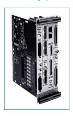
16-channel data acquisition and signal analysis system with T1/E1 interface fits in just four VMEbus slots. System consists of a 4200A MIX Baseboard, a 4257 Dual C40 Coprocessor, a 4259 T1/E1 Transceiver and a Model 4252 16-channel A/D and D/A Converter.
