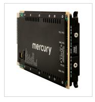
The 5560 is a high-performance, SOSA aligned 3U OpenVPX coprocessor board based on the Xilinx Versal HBM ACAP (Adaptive Compute Acceleration Platform). It serves as an ideal stand-alone processor or as a co-processor for distributed ACAP processing tasks.
