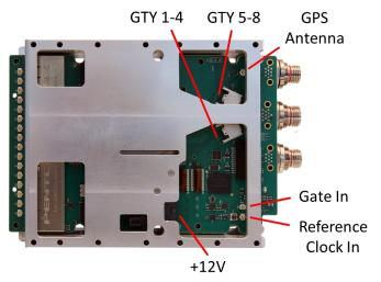
All analog I/O and control and communication interfaces are easily accessible, simplifying connections to other system components.
