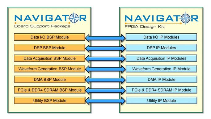
Because all Pentek boards are shipped with a full suite of built-in IP functions and numerous software examples, new applications can be developed by building on the provided software examples or built entirely new with the BSP's extensive libraries. All BSP libraries are provided as C-language source for full access and code transparency.
