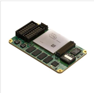
**Quartz® Model 6001 is a high-performance Quartz eXpress Module (QuartzXM) based on the Xilinx Zynq UltraScale+ RFSoc FPGA. The RFSoc FPGA integrates eight RF-class A/D and D/A converters into the Zynq's multiprocessor architecture, creating a multichannel data conversion and processing solution on a single chip.**
