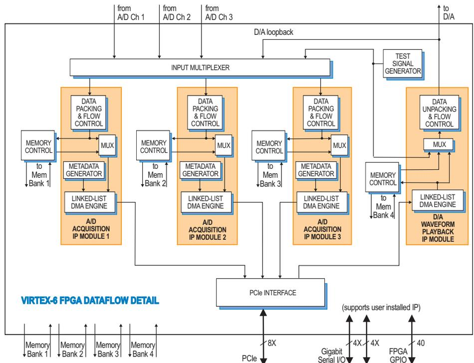
► Each QDRII+ SRAM bank can be up to 8 MB deep and is an integral part of the module's DMA capabilities, providing FIFO memory space for creating DMA packets. For applications requiring deep memory resources, DDR3 SDRAM banks can each be up to 512 MB deep. Built-in memory functions include A/D data transient capture mode and D/A waveform playback mode.
