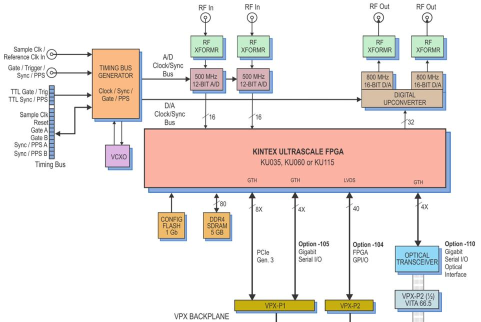
Standard front panel and VPX-P2 connections shown
