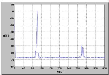
$f_{out} = 100 \text{ MHz}, f_{S} = 800 \text{ MHz}, \text{Interpolation} = 4,$ Internal Clock
