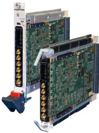
Model 53862 COTS (left) and rugged version
