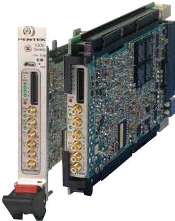
Model 5350 commercial (left) and conduction-cooled version
