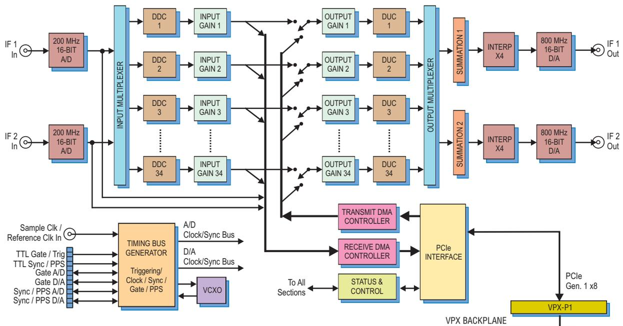
► associated with one of the two D/A converters using a final interpolation factor of  $\times 4$ . After conversion, the IF analog outputs of each D/A can contain signals from any combination of the 34 DUCs.
