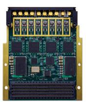
The Flexor® Model 3324 is a multichannel, high-speed data converter FMC. It is suitable for connection to HF or IF ports of a communications or radar system. It includes four 500 MHz, 16-bit A/Ds, four 2 GHz, 16-bit D/As, programmable clocking, and multiboard synchronization for support of larger high-channel-count systems.
