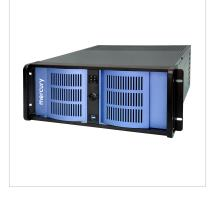
Talon RTR 2742 is a turn-key record and playback system for ultra-wideband analog RF/IF signals. Using two 12-bit, 6.4 GHz A/D converters, this system can achieve sustained recording of 2.4 GHz bandwidth signals at rates up to 6 GBytes per second. It can be configured as a one- or two-channel system and can record real samples or complex I+Q digitally down-converted samples.
