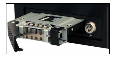
A push of a button unlatches each of the data drives and the OS drive. Drives are mounted on sleds and can be easily transferred to an offload system while the recorder stays in the field.
