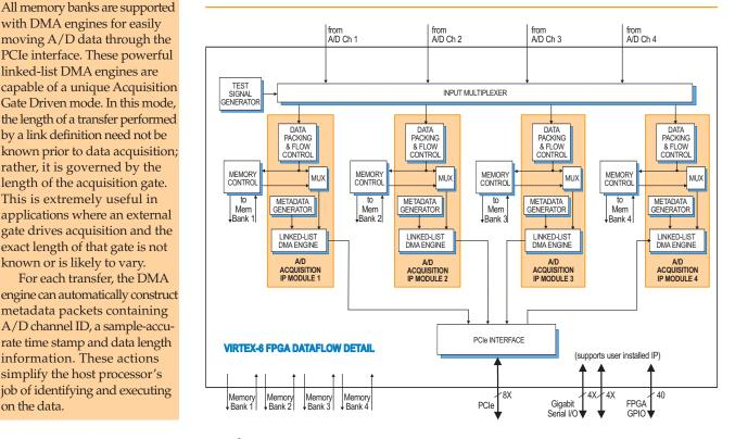
known or is likely to vary. For each transfer, the DMA engine can automatically construct metadata packets containing A/D channel ID, a sample-accurate time stamp and data length information. These actions simplify the host processor's job of identifying and executing on the data.
