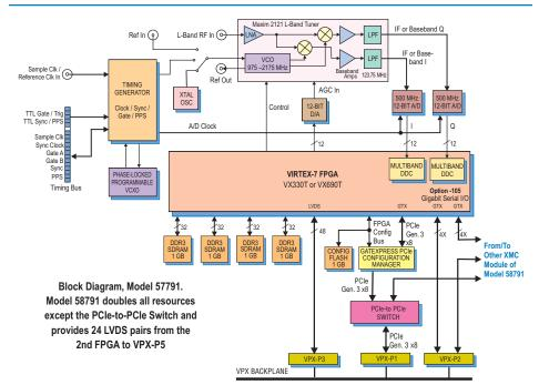
Sample clock synchronization to external system reference
