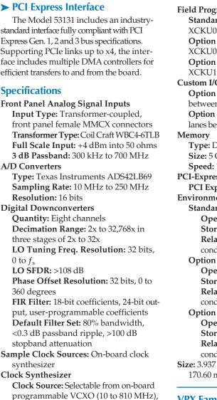
programmable VCXO (10 to 810 MHz), front panel external clock or LVPECL timing bus **Synchronization:** VCXO can be locked to an external 4 to 180 MHz PLL system
