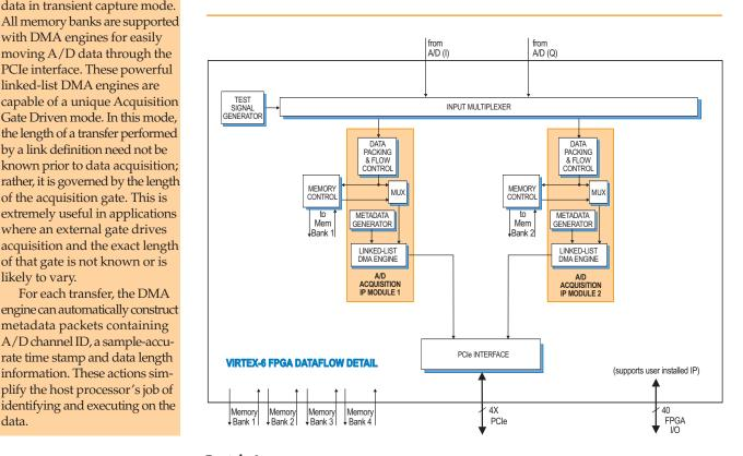
acquisition and the exact length of that gate is not known or is likely to vary. For each transfer, the DMA engine can automatically construct metadata packets containing A/D channel ID, a sample-accurate time stamp and data length information. These actions simplify the host processor's job of identifying and executing on the
