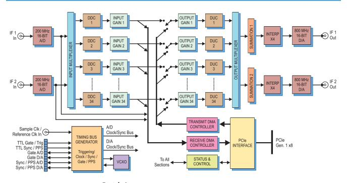
>associated with one of the two D/A converters using a final interpolation factor of x4. After conversion, the IF analog outputs of each D/A can contain signals from any combination of the 34 DUCs.
