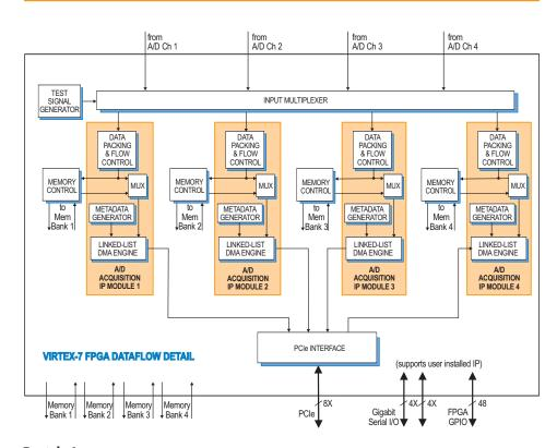
known or is likely to vary. For each transfer, the DMA engine can automatically construct metadata packets containing A/D channel ID, a sample-accurate time stamp and data length information. These actions simplify the host processor's job of identifying and executing on the data.
