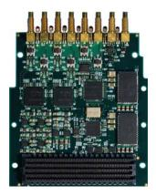
The Flexor® Model 3312 is a multichannel, high-speed data converter FMC module. It includes four 250 MHz, 16-bit A/Ds, two 800 MHz, 16-bit D/As, programmable clocking, and multiboard synchronization for support of larger high-channel-count systems.
