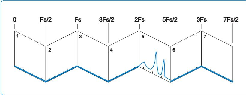
Figure 3. Fan-fold paper showing the spectrum of a bandpass signal such as an IF output.
