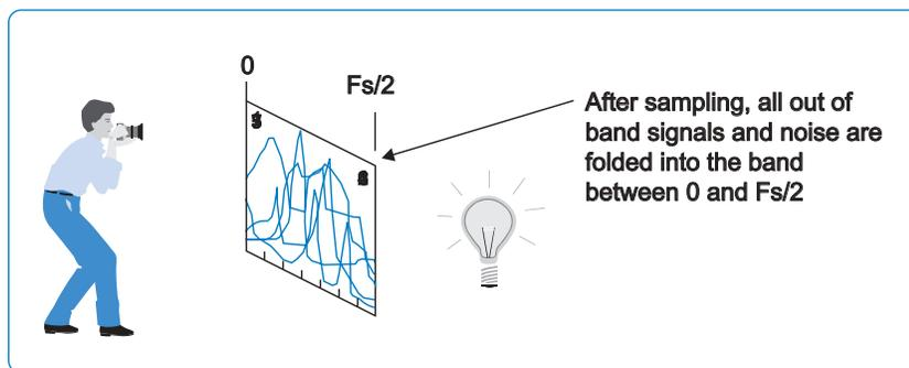
Figure 2. Looking through the collapsed stack reveals the resulting spectrum.
