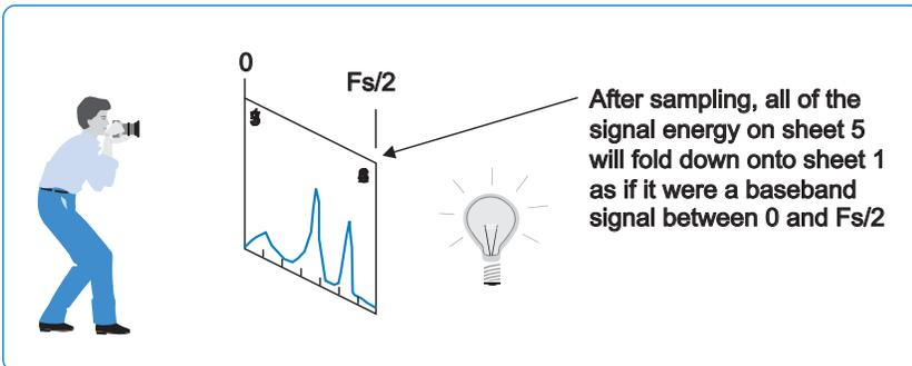
Figure 4. The proper choice of sampling frequency translates the spectrum of the bandpass signal down to baseband.
