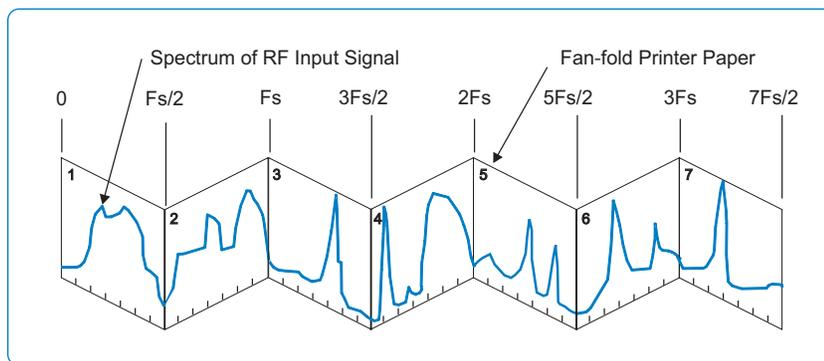
Figure 1. Fan-fold paper showing the spectrum of a RF input signal.
