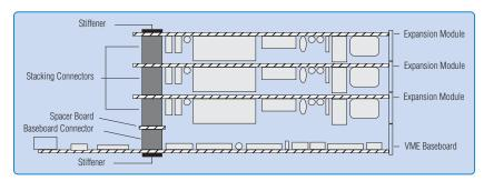
Figure 2. Side view of the MIX stack of Figure 1.
