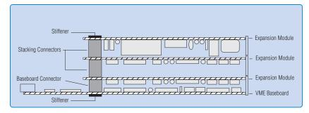
Figure 3. With the first module nesting, it's possible to stack three on a baseboard and still occupy only three card cage slots.
