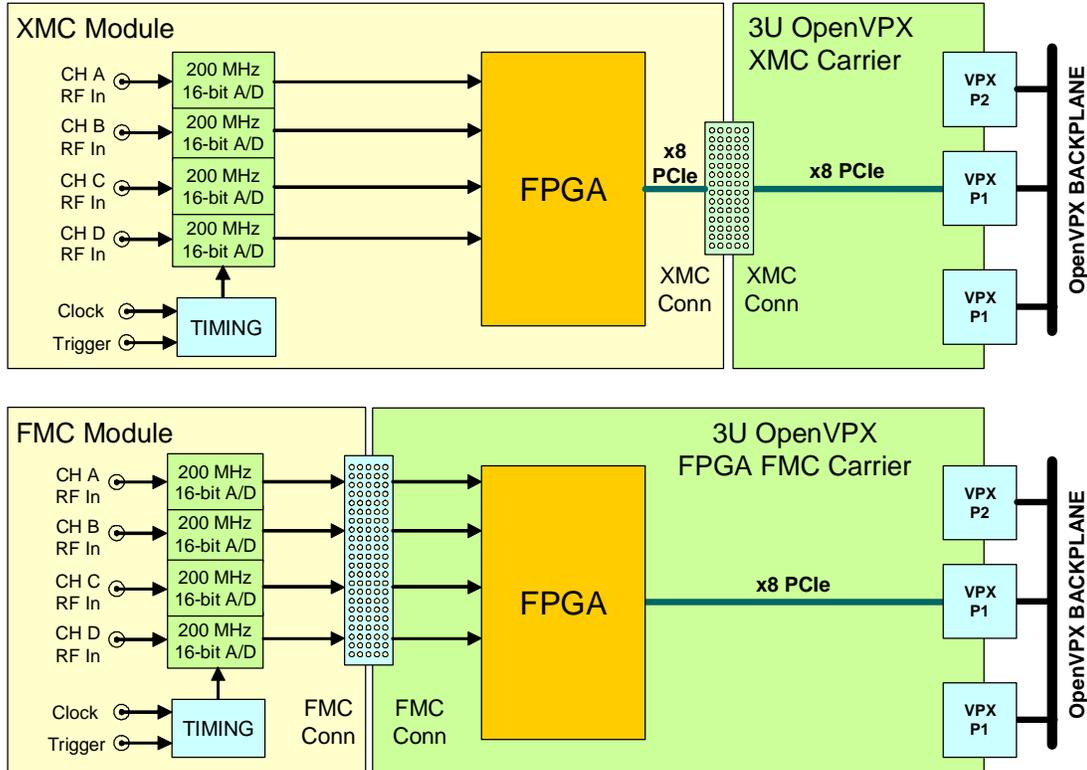
Figure 3. Simplified block diagrams comparing XMC and FMC 4-Channel A/D Software Radio Modules for 3U OpenVPX
