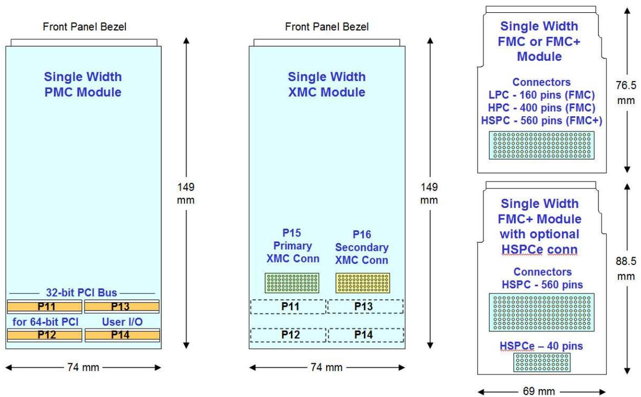
Figure 1. Single PMC, XMC, FMC and FMC+ Module Outline Dimensions & Connectors (drawn to scale, for comparison)
