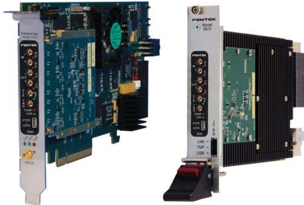
Figure 1: Models 7070-320 PCIe and 5973-320 3U VPX. Two wideband analog I/O modules featuring dual 3 GHz 12-bit A/Ds, dual 2.8 GHz 16-bit D/As, Virtex-7 FPGAs, and DMA engines supporting PCIe Gen 3 x8 PCIe data links to system memory.
