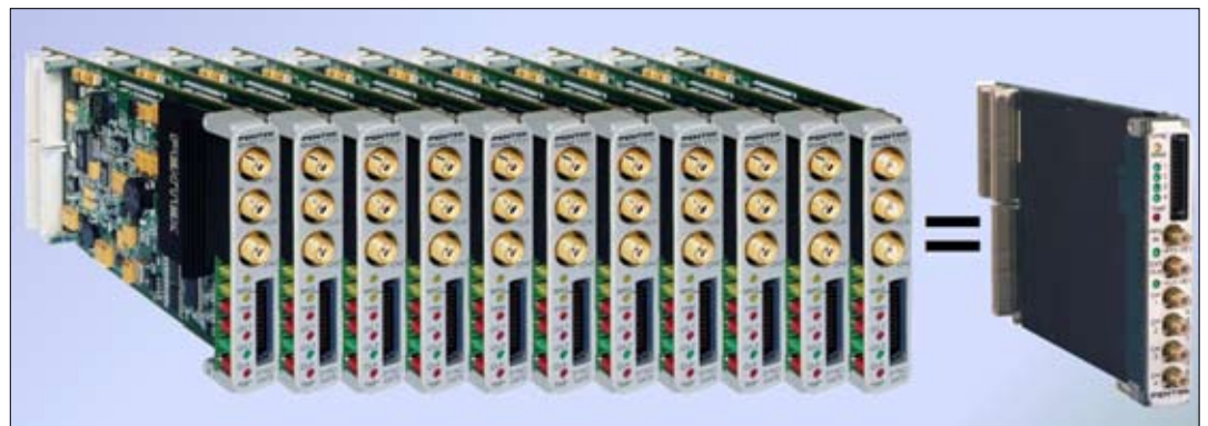
Figure 3: An IP DDC with 174 channels and similar performance to the 4016 can fit in a single Virtex-5 XC5V5X95T FPGA that can be housed on a single PMC.
