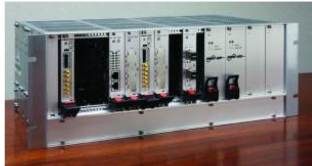
Figure 2. Pentek SPARK 3U VPX Development System with single board computer, VPX switch and software radio modules installed, all ready for software development.
