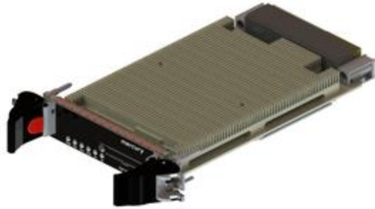
[Figure 1 | Mercury's 3U OpenVPX LDS3517 single-board computer is powered by a Xeon D processor and is SOSA-aligned for maximum interoperability and technology reuse.]
