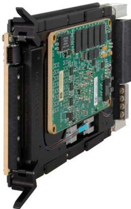
[Figure 3 | Pentek’s newly released Model 5553 Quartz RFSoc 3U VPX SOSA-aligned processor features Gen 3 RFSoc devices with wider signal bandwidths and higher resolution.]
