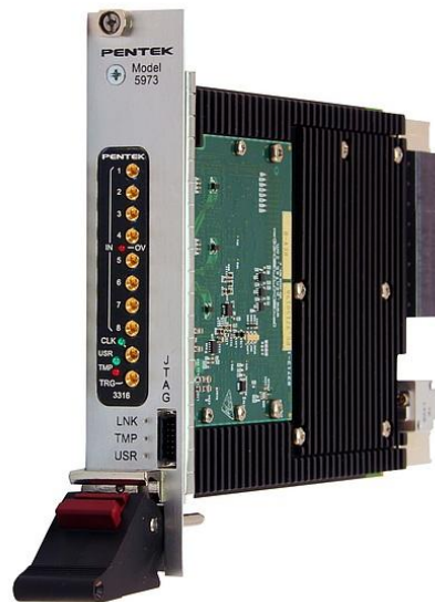
Figure 1: The 5973 3U OpenVPX FMC Carrier board from Pentek enables a high-bandwidth connection between boards mounted in the same chassis or separated over extended distances by leveraging a serial protocol in the FPGA.
