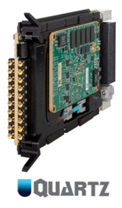
2. Pentek's Model 5950 Quartz system is a 3U OpenVPX board with an UltraScale+ RFSoC Gen 1 chip.
