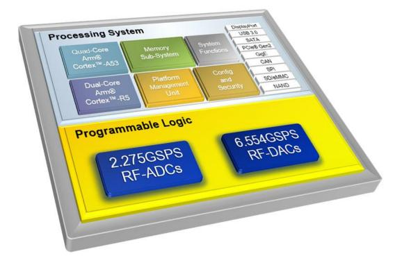
3. The UltraScale+ RFSoC Gen 2 targets 5G with 6.554-Gsample/s RF-DAC and 2.275-Gsample/s RF-ADCs support.
