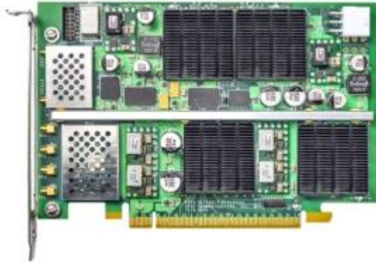
Figure 1. Jeff's Pick is the PVP-7xx family of A-D processing boards from Star Communications. It's scalable from 1 to 4 A/D channels and from 1 to 4 FPGAs (Xilinx high-end Virtex-7 XC7VX485T). Programmable sample rates provide flexibility.
