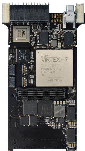
8. Pentek's Model 5973 Flexor Virtex-7 Processor and FMC Carrier board supports the optical VITA 66.4 standard.
