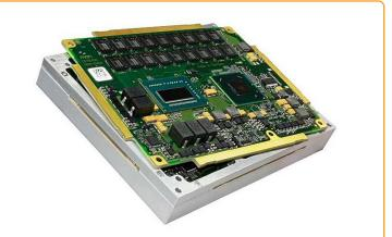
Figure 1. VITA 59 Rugged Com Express module adds thermal tabs to the sides of COM Express boards to pull heat out to a rugged aluminum frame (Courtesy of Men Micro)
