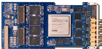
Model 78650: Transceiver, two 500 MHz A/Ds, DUC and two 800 MHz D/As - x8 PCIe
