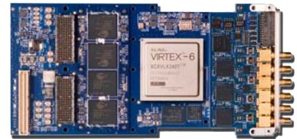
Model 71660: Quad 200 MHz A/D - XMC
