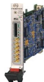
Model 53630: 1 GHz A/D and D/A - 3U VPX
