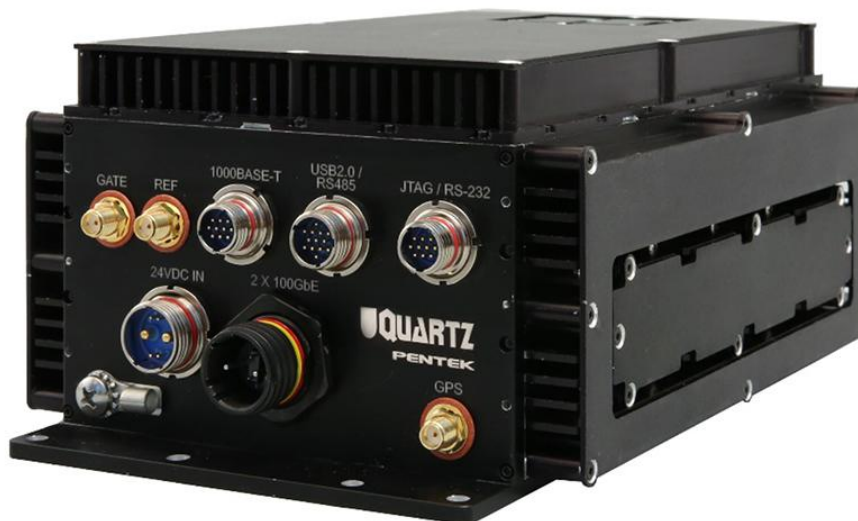
[Figure 2] This RFSoc-based small-form-factor ruggedized subsystem provides eight channels of remote data acquisition and generation, local Arm processor system controller, FPGA fabric for DSP, and dual 100 GbE optical interfaces with VITA-49 data protocol.]
