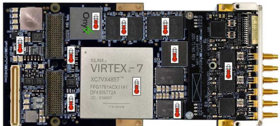
Figure 1. Ten temperature sensors distributed around the Pentek Model 71760 XMC module before mounting it on a PCIe carrier board ensure valid monitoring of cooling effectiveness.
