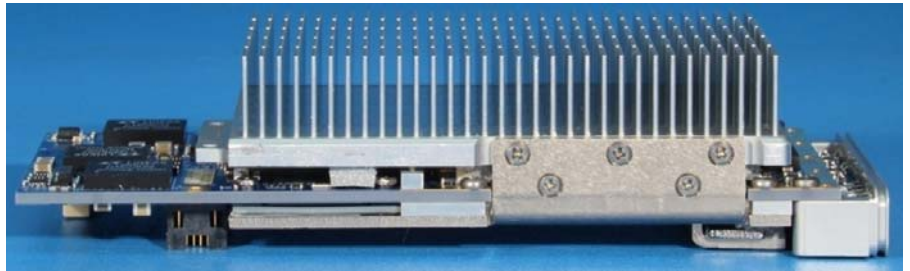
Figure 2. A wrap-around heat sink assembly pulls heat from components on the underside of the XMC module so it isn't trapped by the PCIe carrier card.
