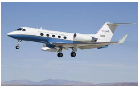
Figure 2. The radar pod is attached to the underside of the aircraft. (Photo courtesy of NASA's Dryden Flight Research Center)
