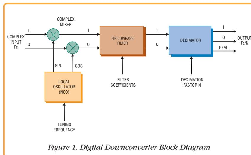
Figure 1. Digital Downconverter Block Diagram
