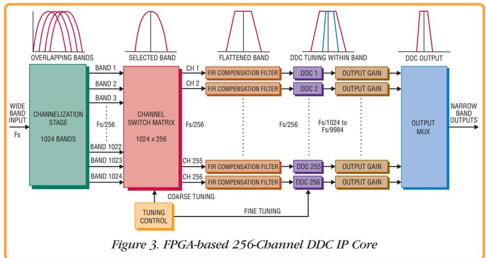
Figure 3. FPGA-based 256-Channel DDC IP Core
