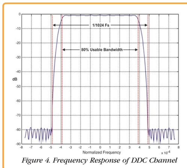
Figure 4. Frequency Response of DDC Channel
